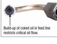
Upgraded oil feed line included to prevent failure, as a clogged line is the most common cause of failure for this application
